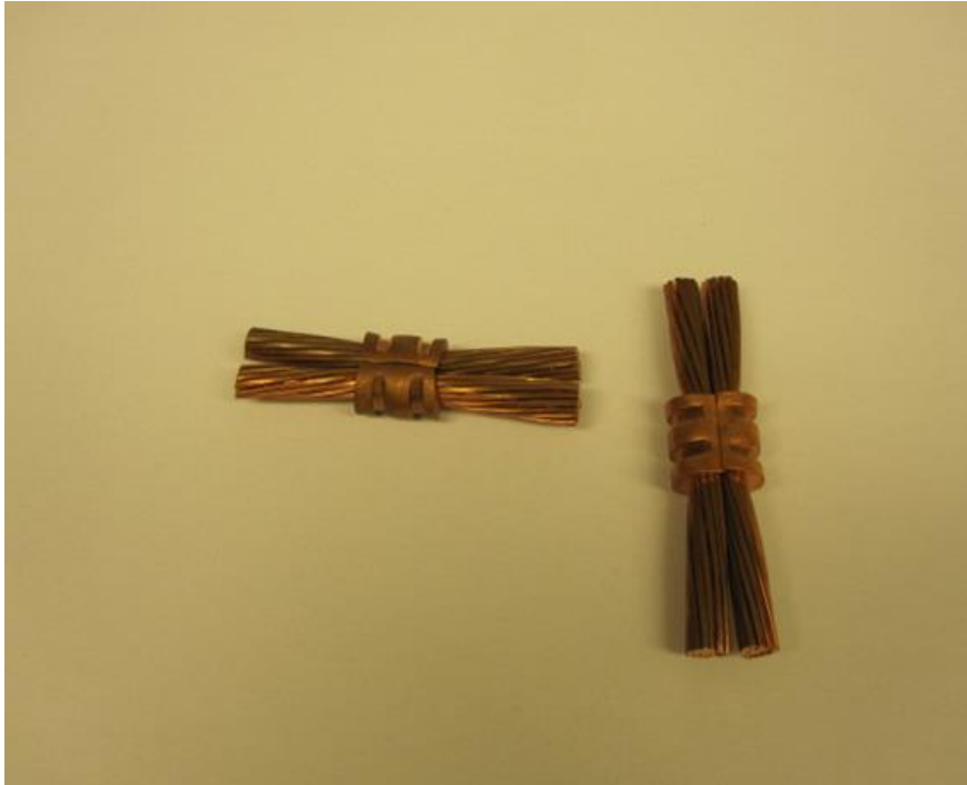
Figure 3: Use of C-type crimp
