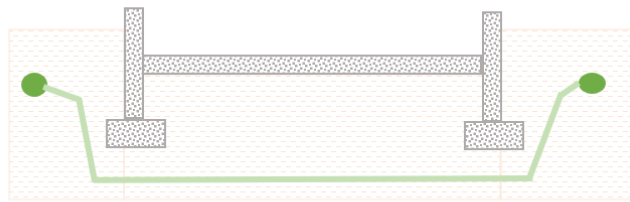
Side view Foundation earth electrode
